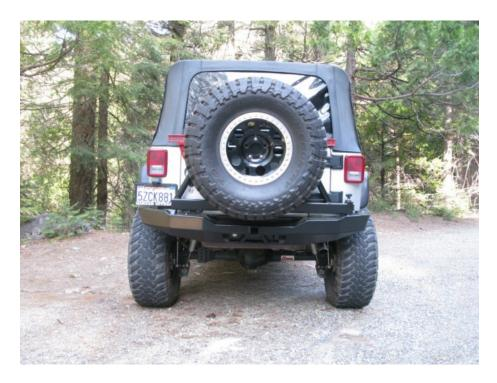
Spindle Bumper w/ Square Frame Style Tire Carrier. (Shown w/ JC4 Cargo Package)
