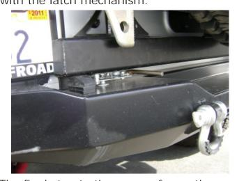
At this point, installation of the round tube tire carrier is complete. Re-check all hardware on the bumper and tire carrier assembly and grease the pivot spindle.
