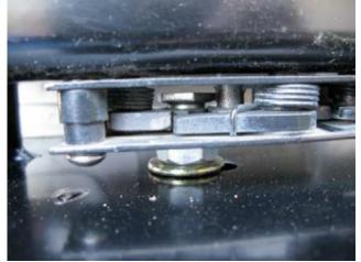
Swing the gate assembly to line up the latch on the tire carrier with the latch pin installed on the bumper. The latch pin is located in a slotted hole for adjustment and can be positioned for smooth operation. Once desired swinging action is achieved, securely tighten the nut on the latch pin and snug the two pivot bolts on the spindle. NOTE: The clamp will not touch in the center. Over-tightening will lift the bumper up off of the bumper causing misalignment with the latch mechanism.
