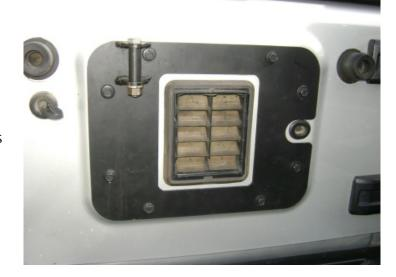
The final step to the sqaure frame tire carrier is the mouting of the upper support plate to the tailgate. Using the factory hardware, securely mount the plate to the tailgate with the pin in the upper left hand corner.
