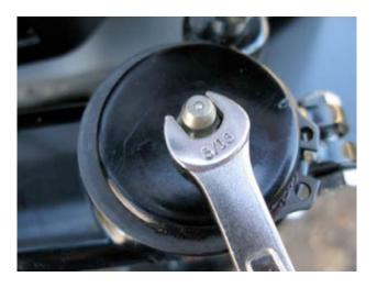
Install snap ring and grease zerk to the spindle assembly. Grease fitting upon completion of tire carrier installation.
